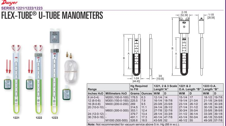
The Series 1221/1222/1223 Flex-Tube® U-Tube Manometers combine the inherent accuracy of the "U" Tube with the durability of tough, long-lasting plastic construction. The columns are made of 0.375" O.D. flexible and shatterproof clear butyrate tubing and are backed by a white scale channel to provide maximum color contrast. These manometers are ideal wherever a portable, direct reading manometer is needed.
