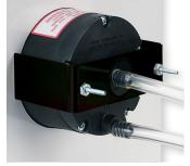
Mounting hardware is supplied with the Minihelic® II gage for panel mounting through a single hole, 2-5/8" (67 mm) in diameter. Panel thickness up to 1/2" (13 mm) can be accommodated with the hardware supplied. If necessary, surface mounting of the gage can be accomplished by means of two 4-40 screws into the tapped mounting bracket stud holes in the rear of the gage. Surface mounting requires clearance holes in the panel for the two pressure taps.
