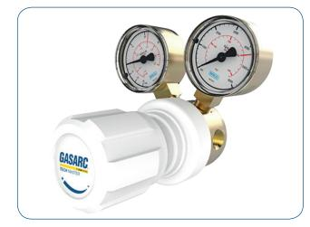
**The Tech Master GPS400** Series single stage diaphragm cylinder regulators are designed for primary pressure gas control of non-corrosive or toxic, technical gases up to grade 4.5 purity (99.995%), on applications where slight variation from decreasing cylinder pressure is acceptable.
