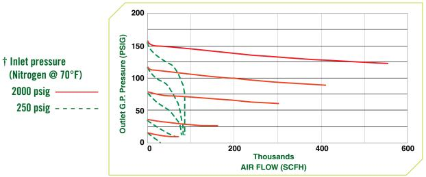
• Tested with outlet valve full open and outlet pressure taken at regulator L.P. gauge port.
